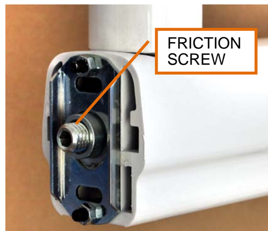
POSITION OF 15 DISK SPRINGS IN FRICTION SCREW 5 GROUPS OF 3
